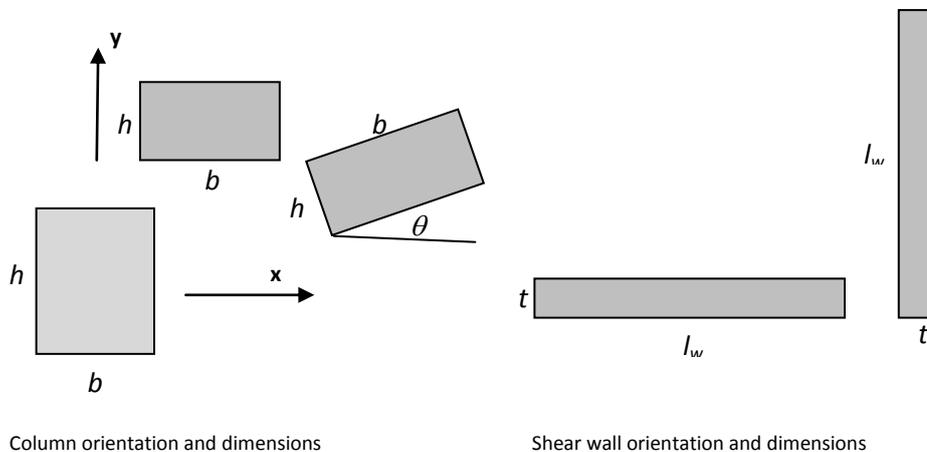
**Figure 6.** Definition of column and shear wall orientations and dimensions
