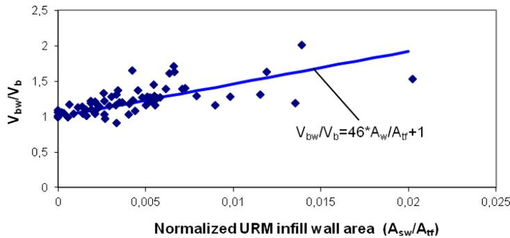
**Figure 7.** The effect of URM infill walls on the base shear capacity of buildings
