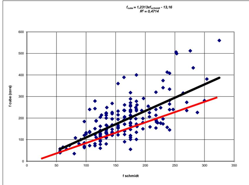
**Figure 4.** Correlation of hammer readings and laboratory tests on samples taken from 200 buildings at Zeytinburnu, Istanbul
